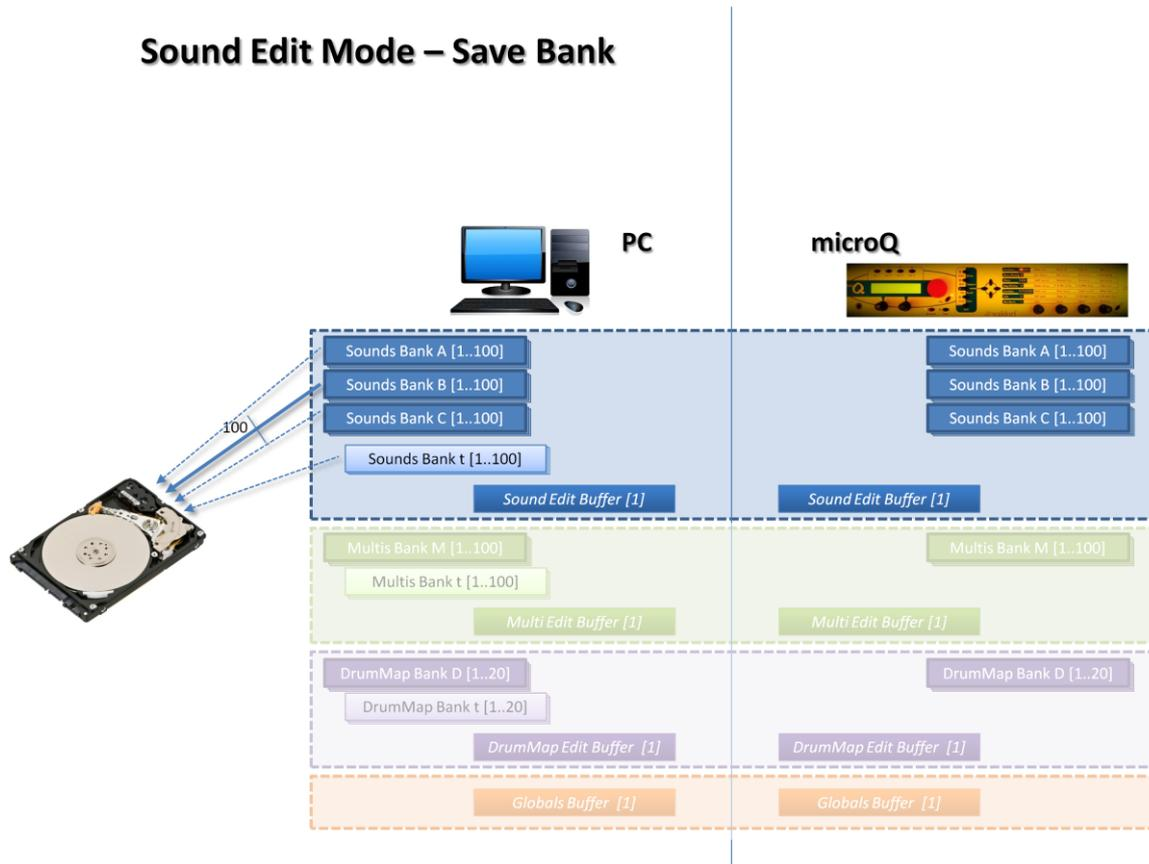
Fig. 25 - The Save Bank Command in Sound Edit Mode: the 100 Sounds from the selected active Bank are stored to a PC file.
