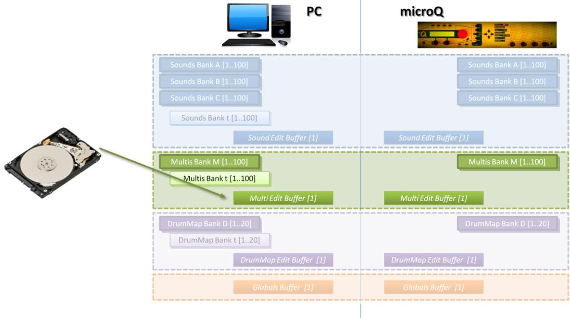
Fig. 34 - Load Edit Buffer in Multi Edit Mode: a PC file can be directly loaded into the Multi Edit Buffer
