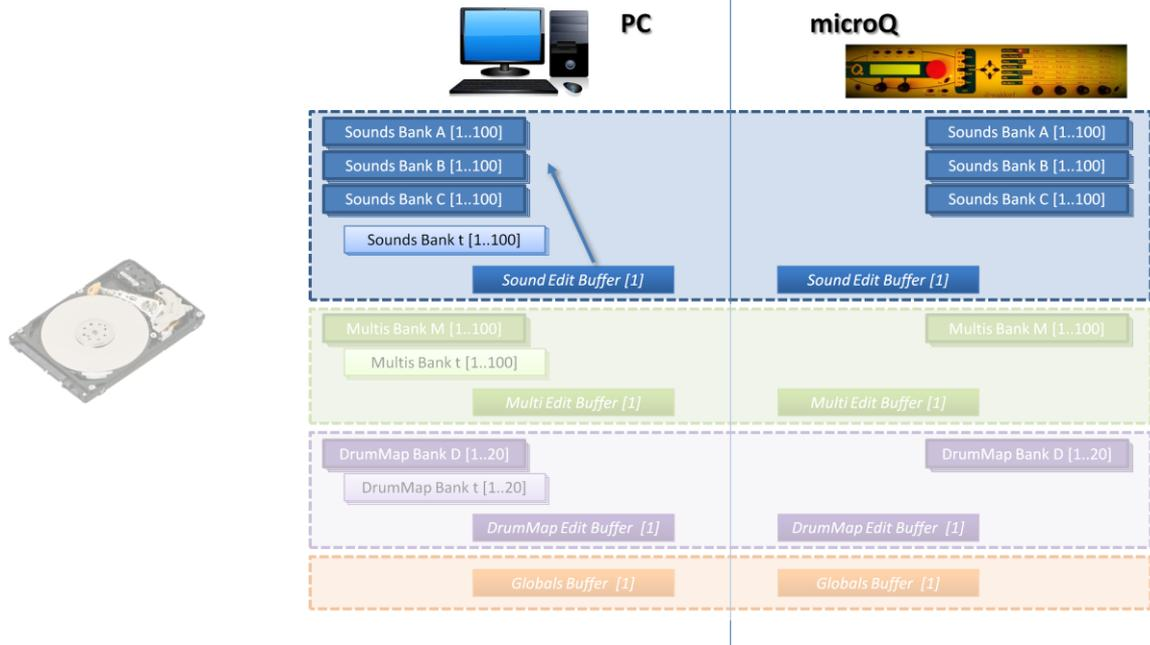
Fig. 30 - Copy Buffer to PC Memory in Sound Edit Mode: the Edit Buffer Sound is copied into one of the memory locations of the Bank A, B, C, or t.
