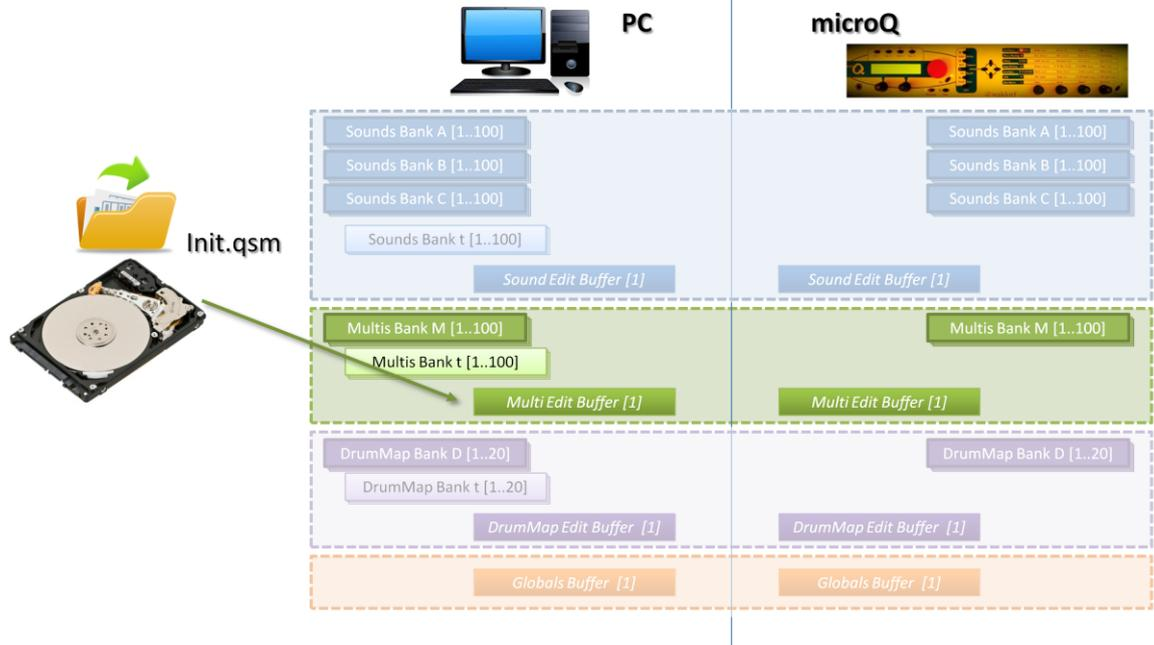
Fig. 40 – Initialization of the Multi Edit Buffer: the file INIT.QSM is loaded and copied into the Edit Buffer
