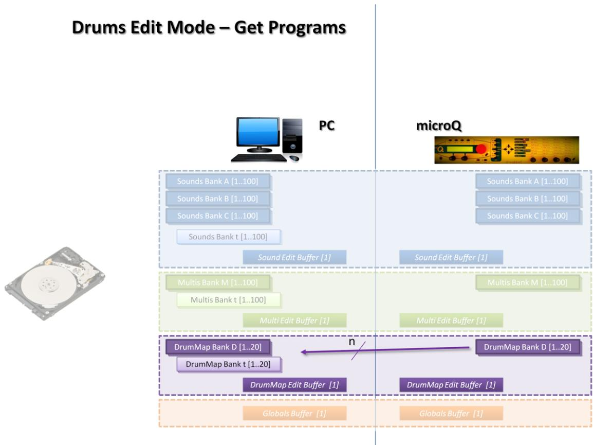
Fig. 51 - Get Programs in DrumMap Edit Mode: the content of a range of contiguous Drums on the Waldorf microQ is copied into the PC Editor memory, starting from a user defined location.
