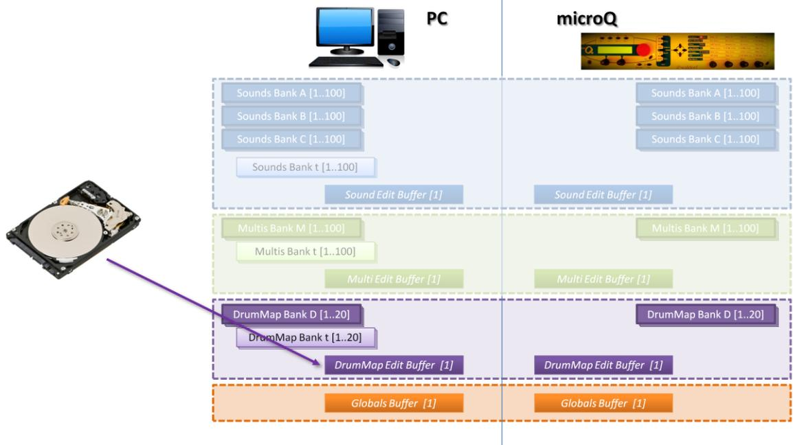
Fig. 35 - Load Edit Buffer in Drums Edit Mode: a PC file can be directly loaded into the Drums Edit Buffer
