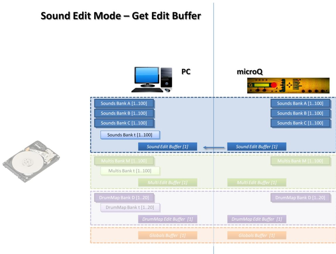
Fig. 42 - Get Edit Buffer in Sound Edit Mode: the content of the Waldorf microQ Sound Edit Buffer is copied into the corresponding PC Editor buffer.
