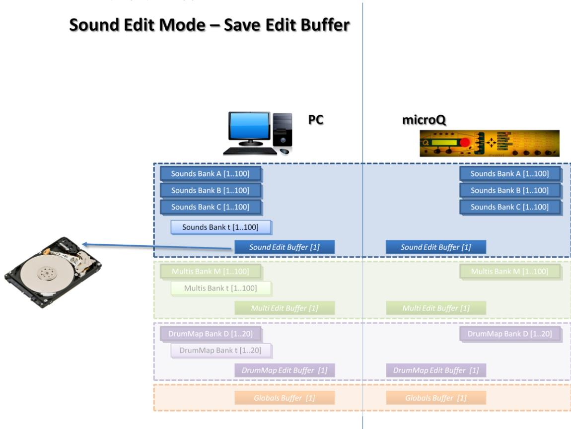
Fig. 36 - Save Edit Buffer in Sound Edit Mode: its content can be stored to a PC file.
