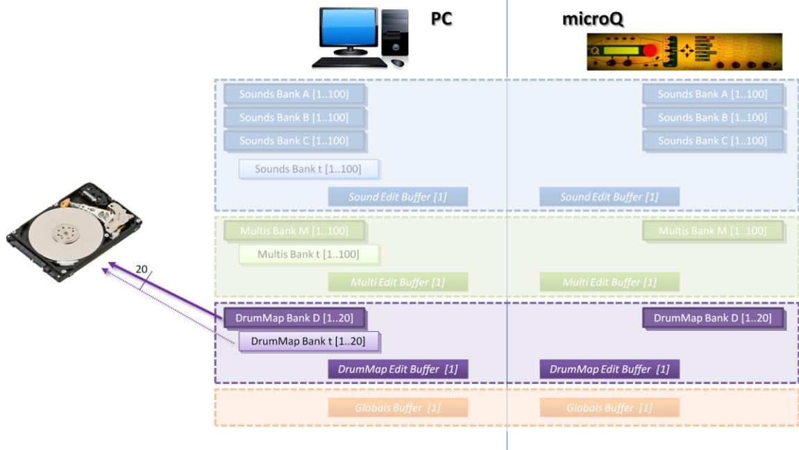
Fig. 27 - The Save Bank Command in DrumMap Edit Mode: the 20 DrumMaps from the active Bank are stored to a PC file.
