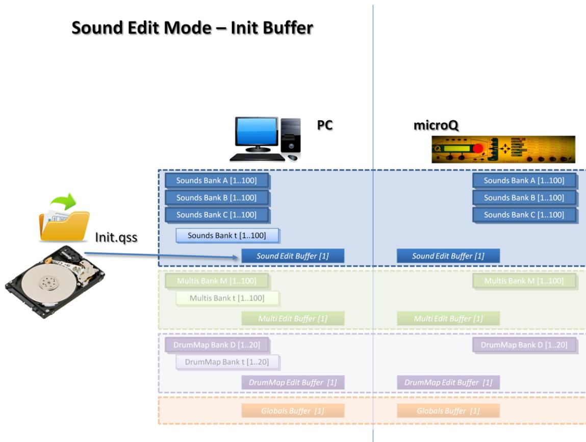
Fig. 39 – Initialization of the Sound Edit Buffer: the file INIT.QSS is loaded and copied into the Edit Buffer
