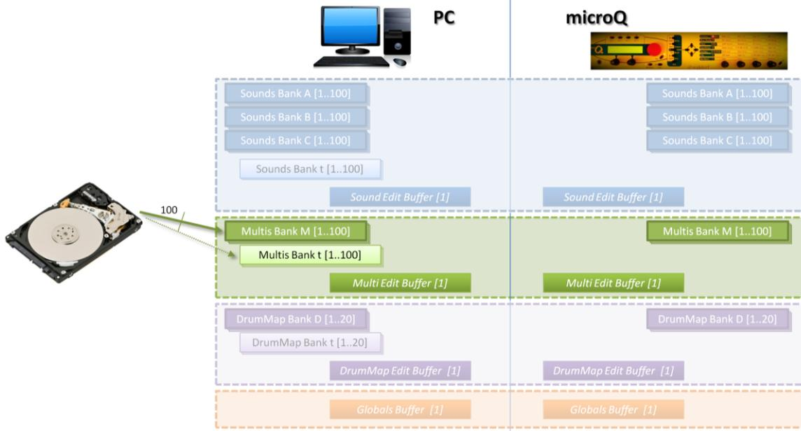
Fig. 23 - The Load Bank Command in Multi Edit Mode: 100 Multis are loaded from a PC file and copied into the active Bank (Bank M in the figure)
