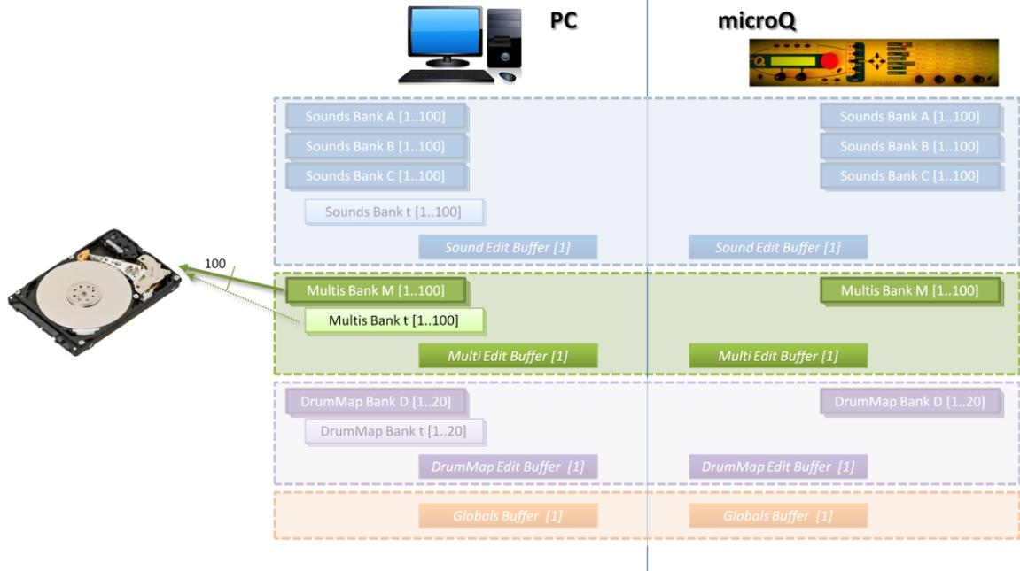
Fig. 26 - The Save Bank Command in Multi Edit Mode: the 100 Multis from the selected active Bank are stored to a PC file.
