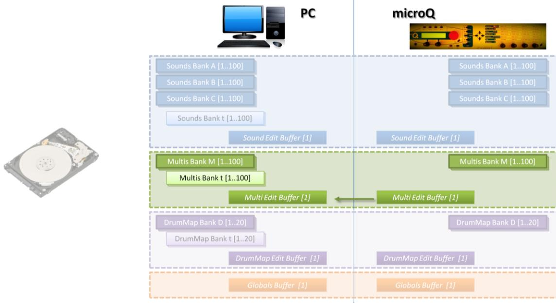
Fig. 43 - Get Edit Buffer in Multi Edit Mode: the content of the Waldorf microQ Multi Edit Buffer is copied into the corresponding PC Editor buffer.
