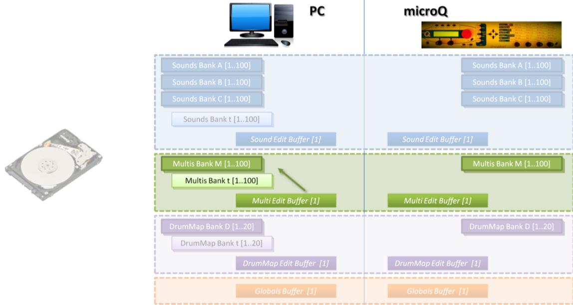
Fig. 31 - Copy Buffer to PC Memory in Multi Edit Mode: the Edit Buffer Multi is copied into one of the memory locations of the Bank M or t.
