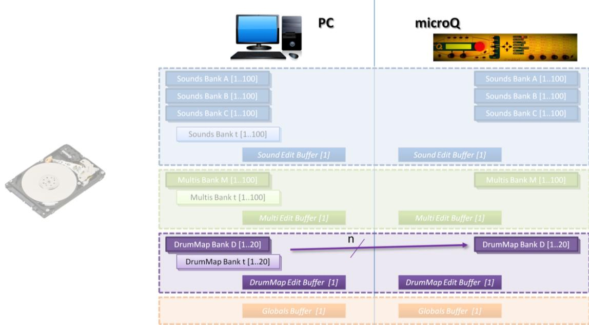
Fig. 54 - Set Programs in Drum Map Edit Mode: the content of a range of contiguous DrumMaps on the PC Editor is copied into the Waldorf microQ memory, starting from a user defined location.
