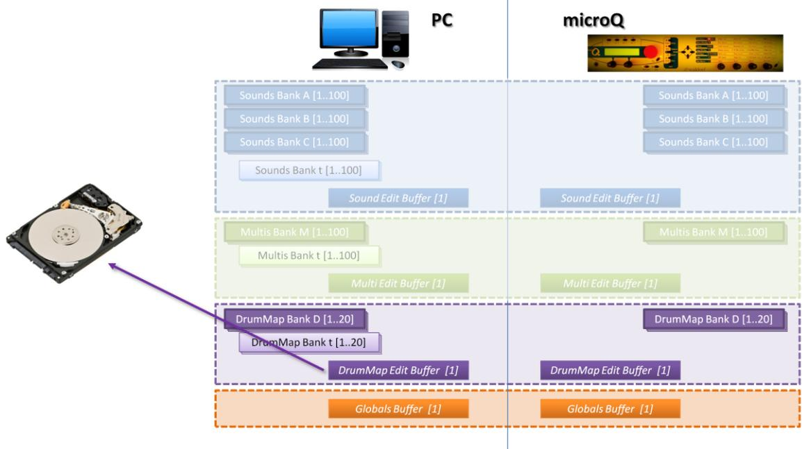
Fig. 38 - Save Edit Buffer in Drums Edit Mode: its content can be stored to a PC file.
