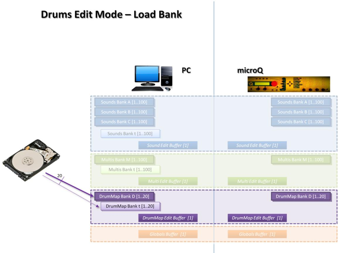
Fig. 24 The Load Bank Command in DrumMap Edit Mode: 20 DrumMaps are loaded from a file and copied into the active Bank (Bank D in the figure)
