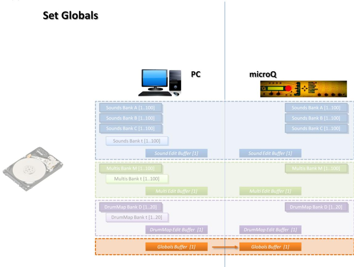
Fig. 56 - Globals buffer from thePC Editor is copied onto the corresponding buffer on the Waldorf microQ
