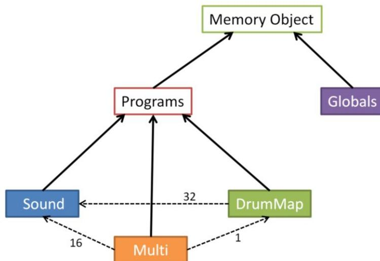
Fig. 1 - Memory Object hierarchy of the Waldorf microQ and the microQ PC Editor
