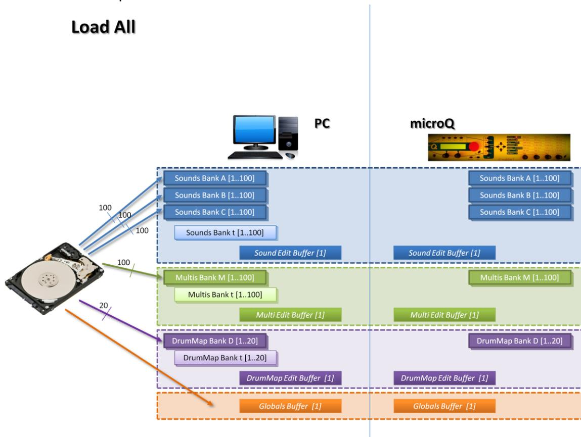
Fig. 28 - The Load All command: 300 Sounds, 100 Multis, 20 DrumMaps and the Globals Buffer are loaded from a PC file.
