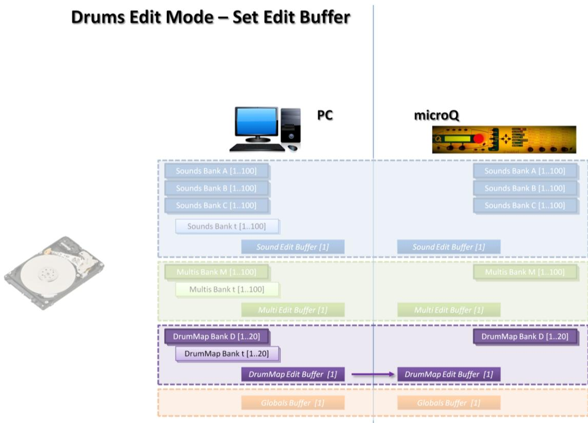
Fig. 47 - Set Edit Buffer in DrumMap Edit Mode: the content of the PC Editor Drums Edit Buffer is copied into the corresponding Waldorf microQ buffer.
