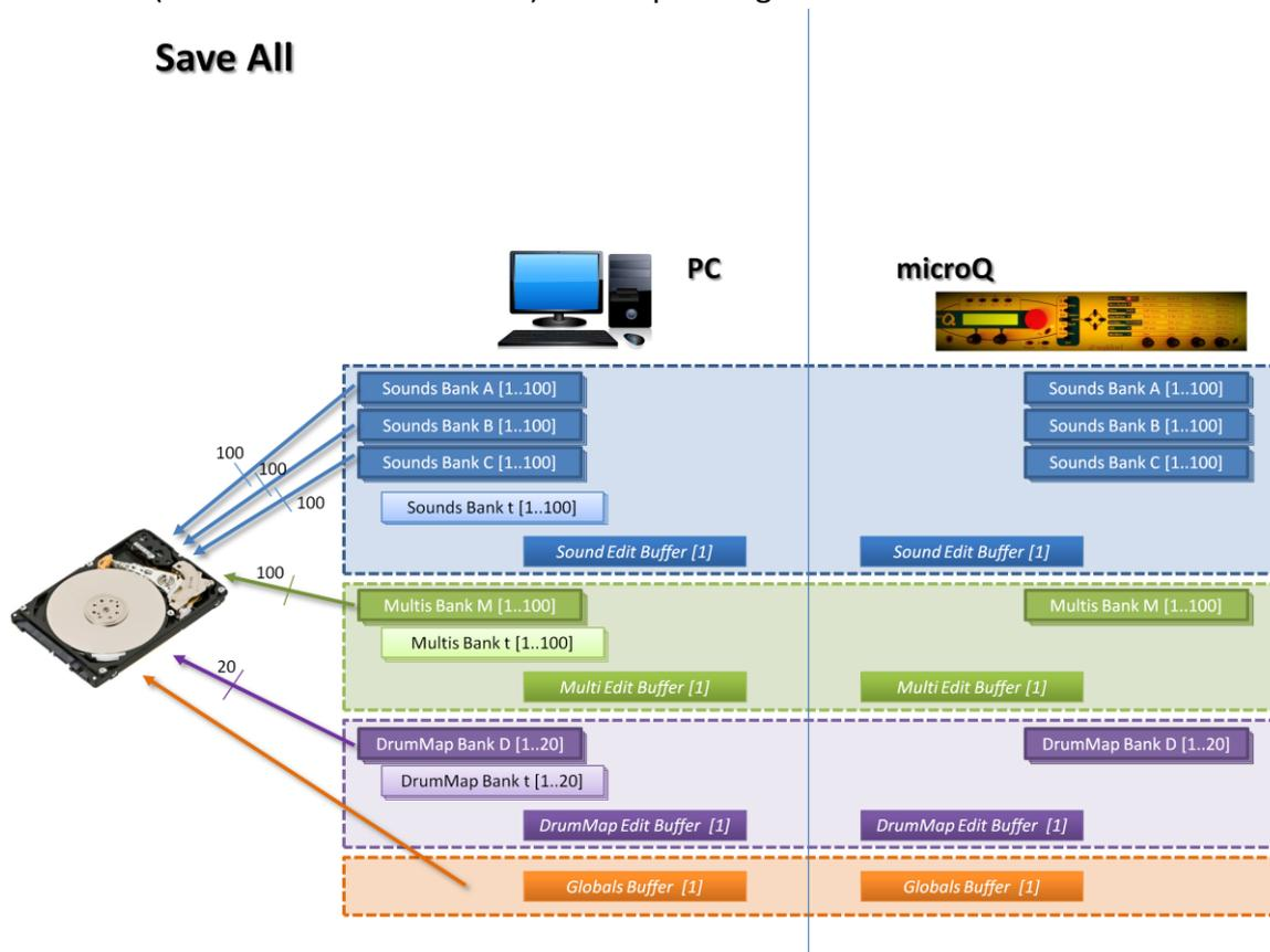
Fig. 29 - The Save All command: 300 Sounds, 100 Multis, 20 DrumMaps and the Globals Buffer are stored into a PC file.
