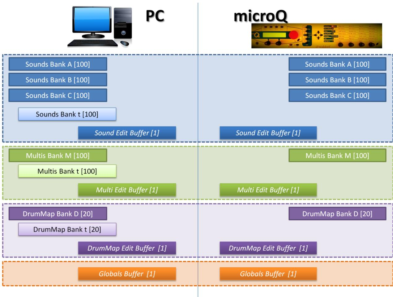
Fig. 3 - Memory blocks of the objects handled by the PC Editor (left) and the Waldorf microQ device
