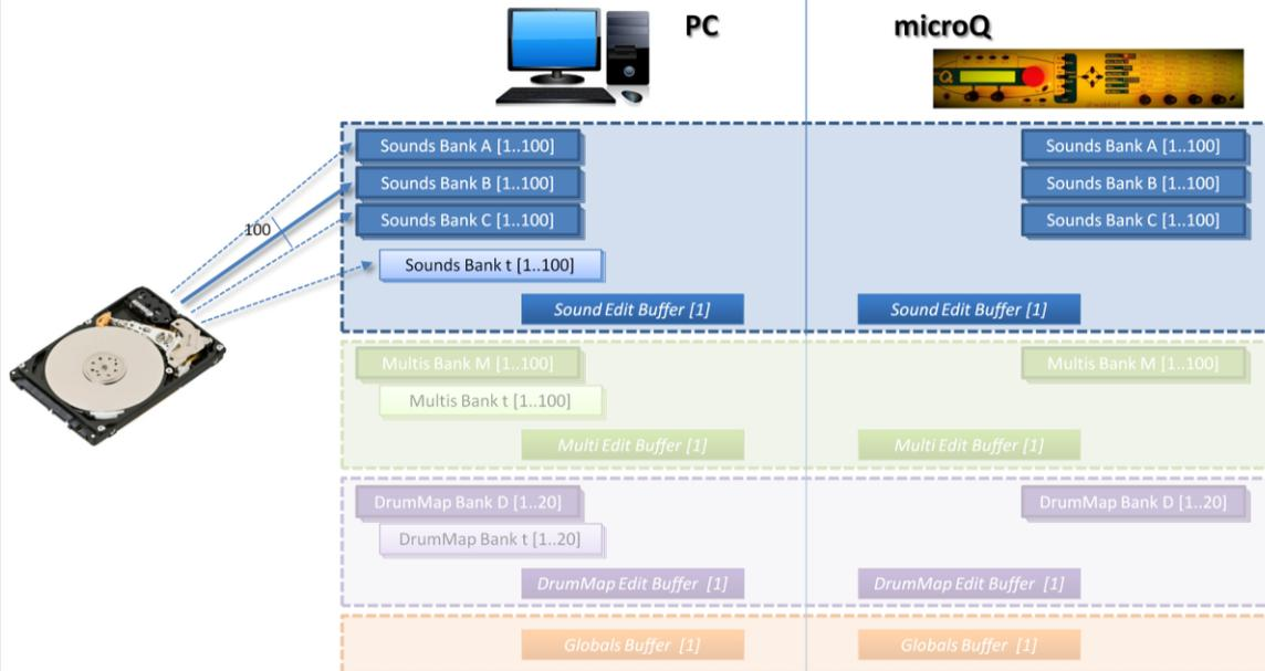
Fig. 22 - The Load Bank Command in Sound Edit Mode: 100 Sounds are loaded from a PC file and copied into the active Bank (Bank B in the figure)
