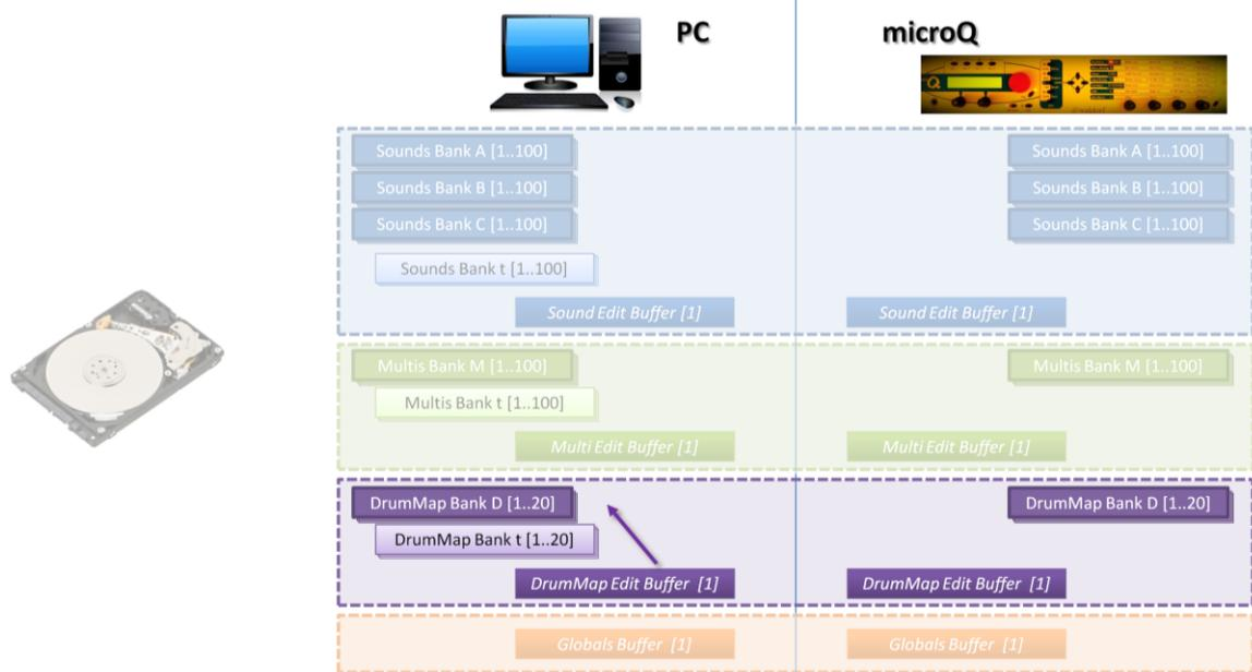
Fig. 32- Copy Buffer to PC Memory in Multi Edit Mode: the Edit Buffer Multi is copied into one of the memory locations of the Bank D or t.
