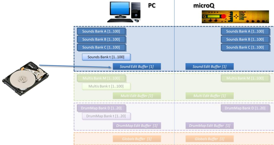
Fig. 33 - Load Edit Buffer in Sound Edit Mode: a PC file can be directly loaded into the Sound Edit Buffer
