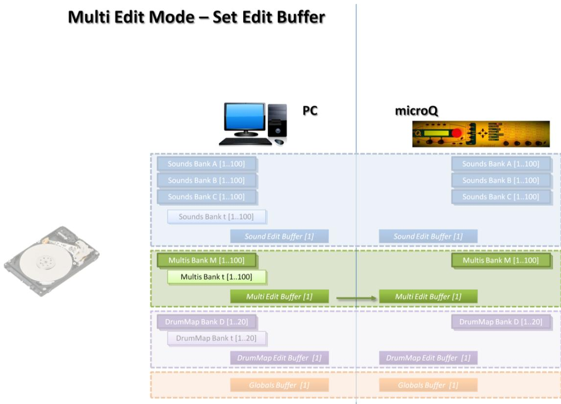
Fig. 46 - Set Edit Buffer in Multi Edit Mode: the content of the PC Editor Multi Edit Buffer is copied into the corresponding Waldorf microQ buffer.
