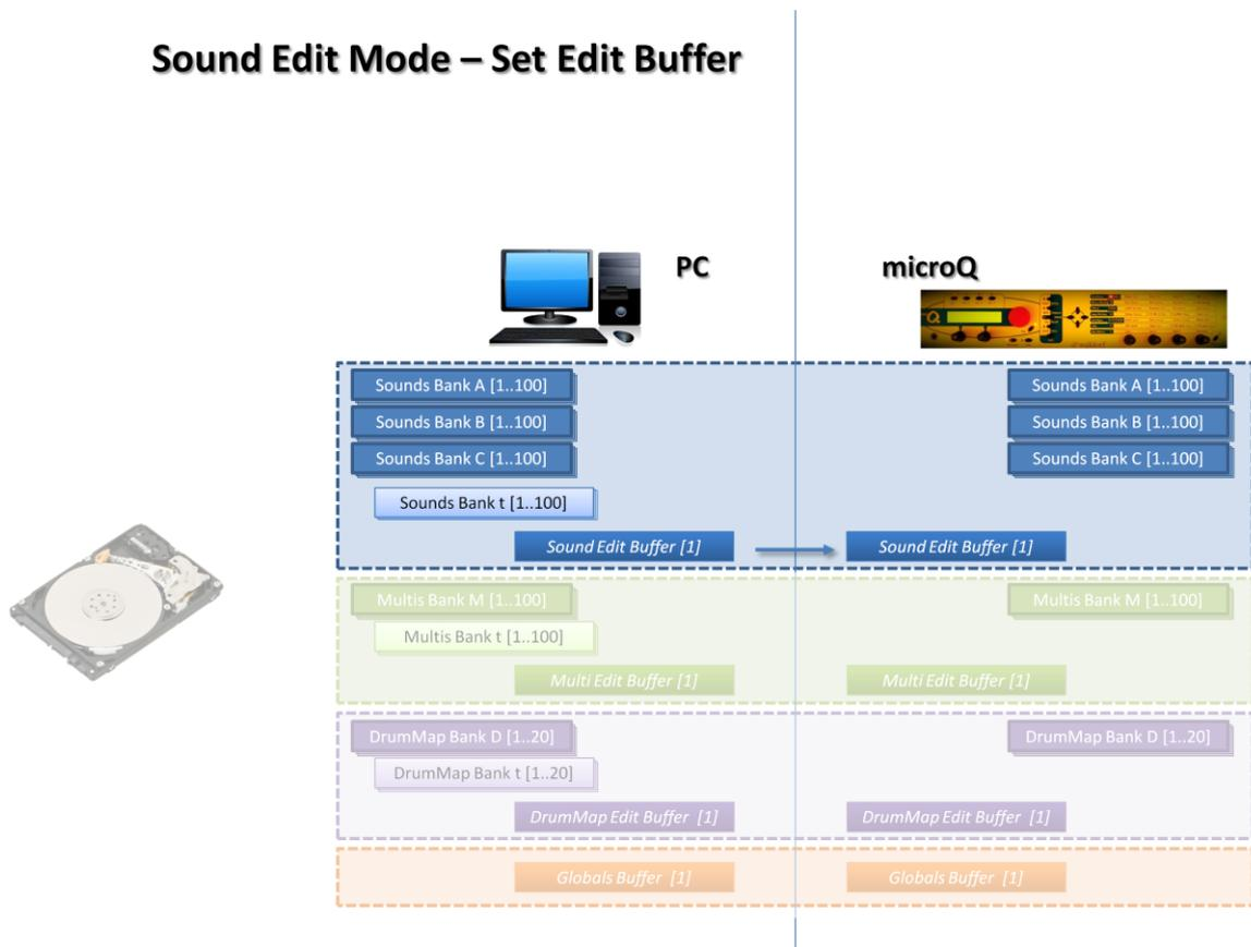
Fig. 45 - Set Edit Buffer in Sound Edit Mode: the content of the PC Editor Sound Edit Buffer is copied into the corresponding Waldorf microQ buffer.
