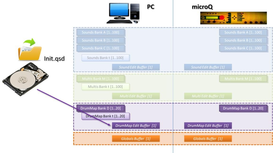
Fig. 41 – Initialization of the Drum Map Edit Buffer: the file INIT.QSD is loaded and copied into the Edit Buffer
